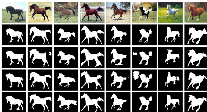
Fig. 2. Segmentation examples on Weizmann horse. 1st row: test images; 2nd row: ground truth; 3rd row: segmentation results produced by SVM based CRF learning with bag-of-words feature; 4th row: segmentation results produced by SSVM based CRF learning with unsupervised feature learning; 5th row: segmentation results produced by SSVM based CRF learning with the 6th layer CNN features.
