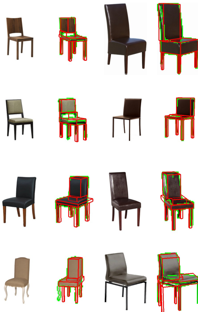
Figure 5.12: Learning the structure of a chair object. Model fitting is done jointly for the fifteen images in the training set using contiguous blocks to represent the structure. The fits for the training examples is shown by the blocks drawn in red. Detected edge points are shown in green.
